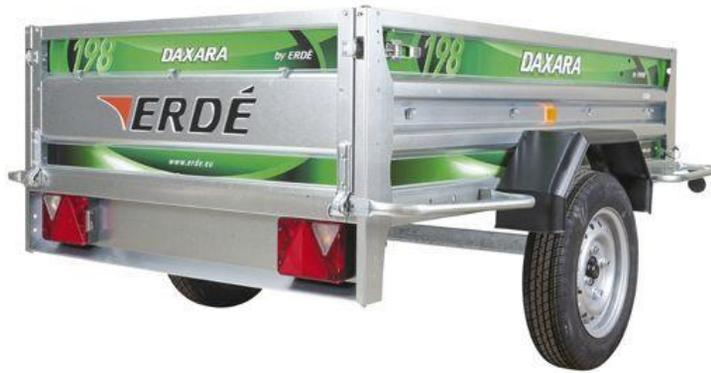
The Daxara 198 is an unbraked 6' x 3' 9" single axle trailer, constructed with profiled galvanised pressed steel sides. It has a gross vehicle weight of 750kgs and can carry up to 585kgs.
