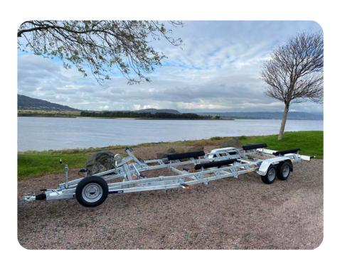
If your hull shape isn't suitable for a roller system or if you require more weight capacity, the Dipper and Big Dipper range is for you. Fully adjustable to suit many shapes and sizes of boats from 4.5m to 9m. Carpeted bunks and keel rollers give maximum hull and keel support. The option of an inboard propeller cut out frame is available for under hull propeller boats.
